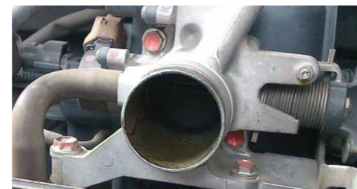
BEFORE (Throttle body condition after 60,000 km)
