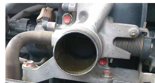
BEFORE (Throttle body condition after 60,000 km)
